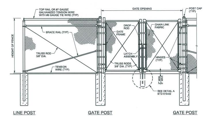
24' x 6' High galvanized double swing gates with locking assembly
